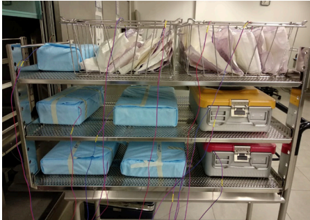
Figure 4: Example of a hospital load configuration with different medical devices and sterile barriers
